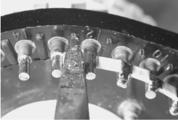
Fig. 7.9 Soldering surface mount resistors using a jig. Note that the next soldered joint will solder one end of the new resistor and the (previously unsoldered end) of the previous resistor
