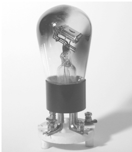
Fig. 4.25 P215 directly heated oxide-coated cathode valve
